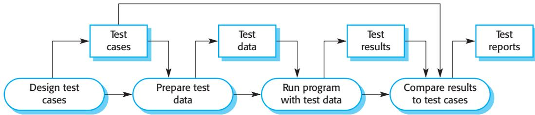
Figure 23.2 A model of the software testing process
