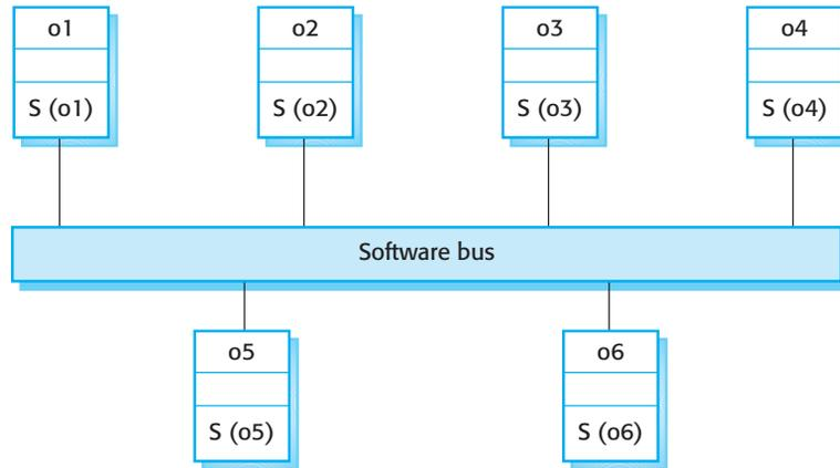
Its role is to provide a seamless interface between objects. It provides a set of services that allow objects to communicate and to be added to and removed from the system. I discuss object request brokers in Section 12.3.1.
