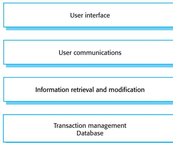
Figure 13.7 The architecture of the LIBSYS system
