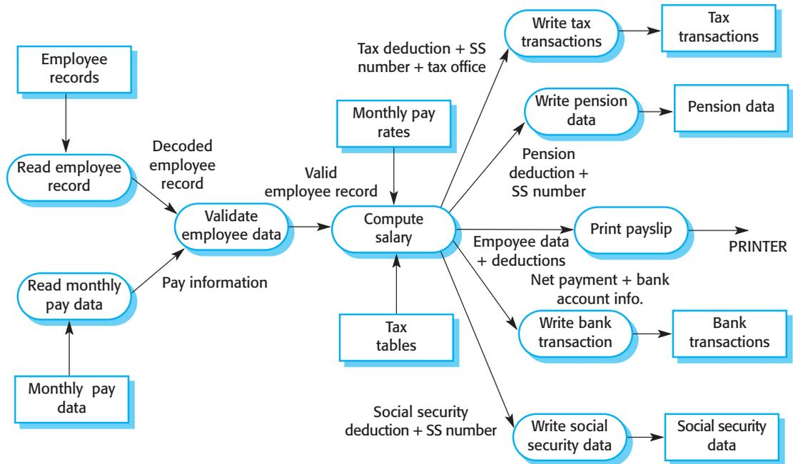
Figure 13.2 Data-flow diagram of a payroll system
