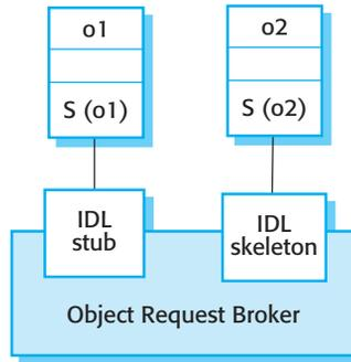
Object request brokers are not usually implemented as separate processes but are a set of libraries that can be linked with object implementations. Therefore, in a distributed system, each computer that is running distributed objects will have its own object request broker. This will handle all local invocations of objects. However, a request made for a service that is to be provided by a remote object requires inter-ORB communications.
