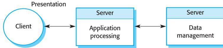
Figure 12.8 The distribution architecture of an Internet banking system
