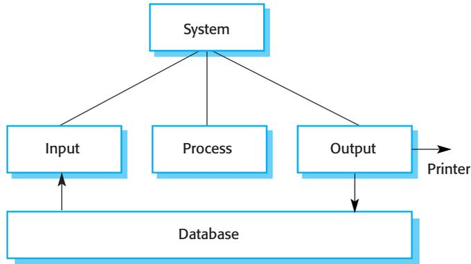
2. A processing component may take a transaction from a queue (input), perform some computations on the data and create a new data record recording the results of the computation (process), then queue this new record for printing (output). Sometimes the processing is done within the system database and sometimes it is a separate program.
