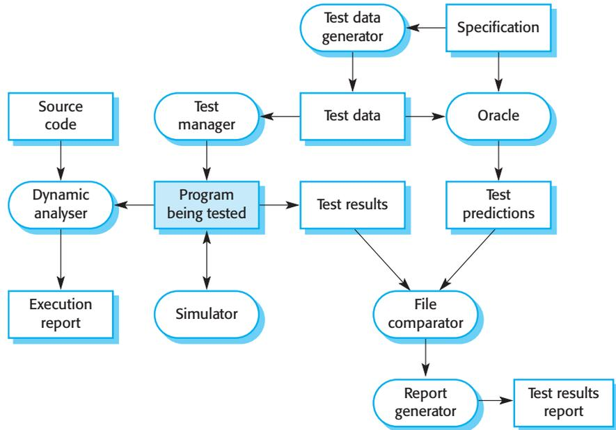
A software testing workbench is an integrated set of tools to support the testing process. In addition to testing frameworks that support automated test execution, a workbench may include tools to simulate other parts of the system and to generate system test data. Figure 23.17 shows some of the tools that might be included in such a testing workbench:
