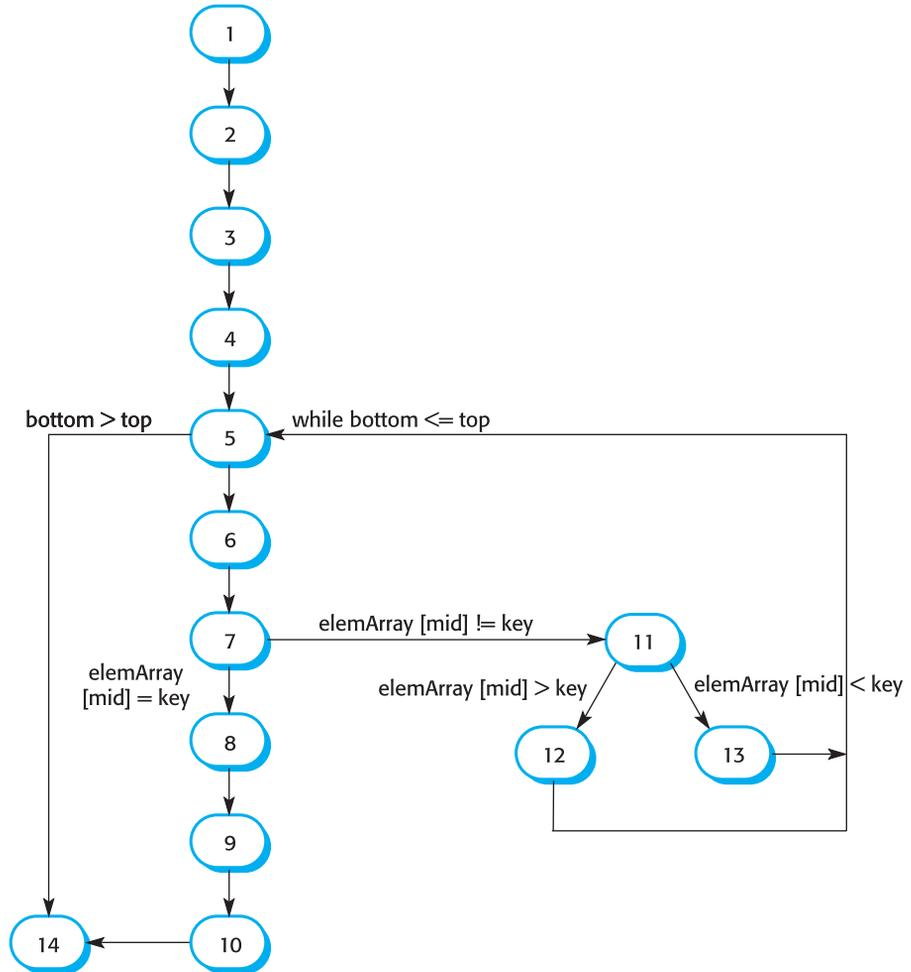
The flow graph for the binary search procedure is shown in Figure 23.16 where each node represents a line in the program with an executable statement. By tracing the flow, therefore, you can see that the paths through the binary search flow graph are:
