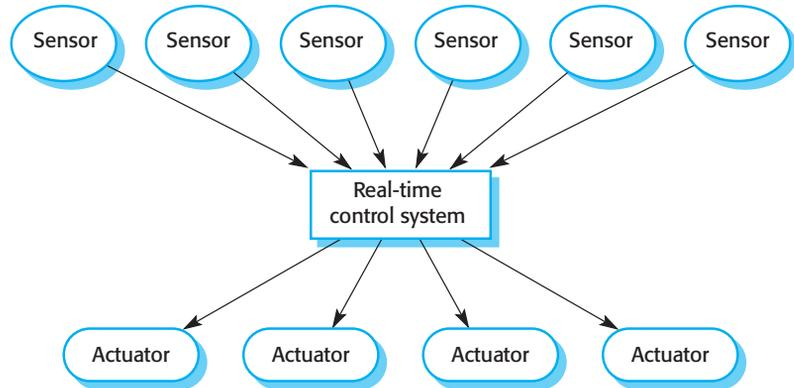
handled by the system. This sensor-system-actuator model of an embedded real-time system is illustrated in Figure 15.1.
