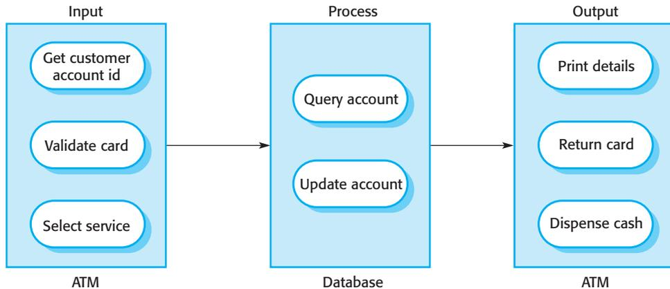
Figure 13.4 The software architecture of an ATM
