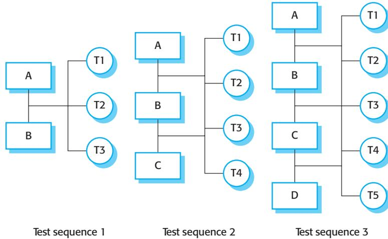
configuration and test this system. You then add components to this minimal configuration and test after each added increment.
