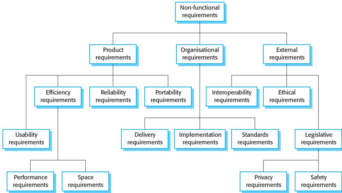
Figure 6.3 Types of non-functional requirements
