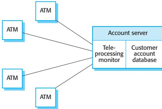
This ATM distributed system is illustrated in Figure 12.6. Notice that the ATMs do not connect directly to the customer database but to a teleprocessing monitor. A teleprocessing monitor or transaction manager is a middleware system that organises communications with remote clients and serialises client transactions for processing by the database. Using serial transactions means that the system can recover from faults without corrupting the system data.
