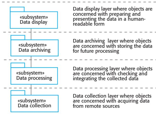
automatically collected meteorological data. The detailed requirements for such a weather mapping system would take up many pages. However, an overall system architecture can be developed from a relatively brief system description:
