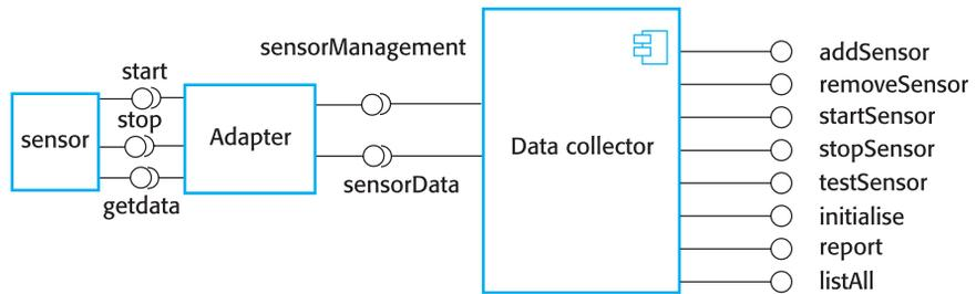
sensor interface. I anticipated that an adaptor would always be used to connect the data collector to a specific sensor interface.
