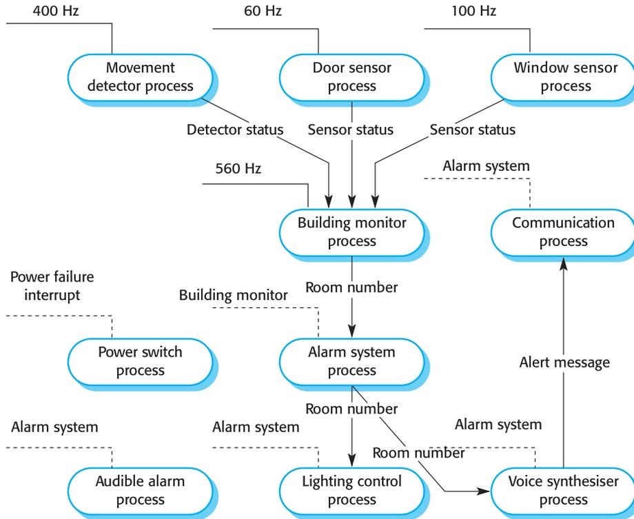
Figure 15.8 Process architecture of the intruder alarm system
